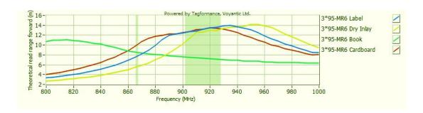
Sensitivity&Read Range Test power: 4W EIRP
